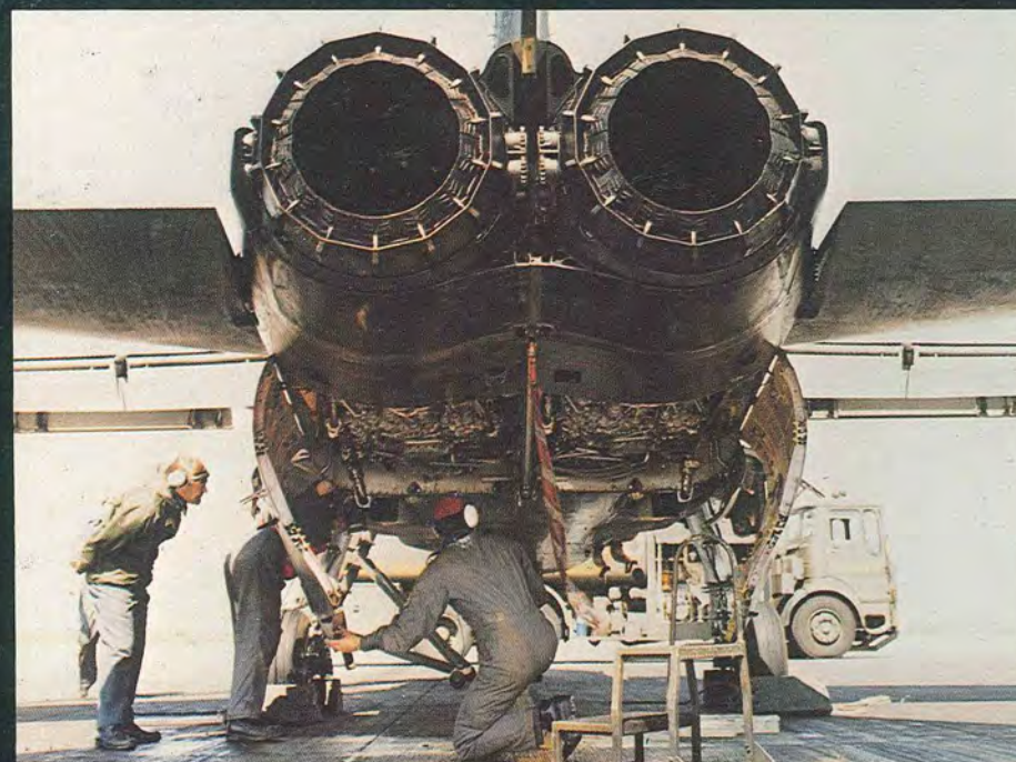
Access to all engine accessories through two large doors
