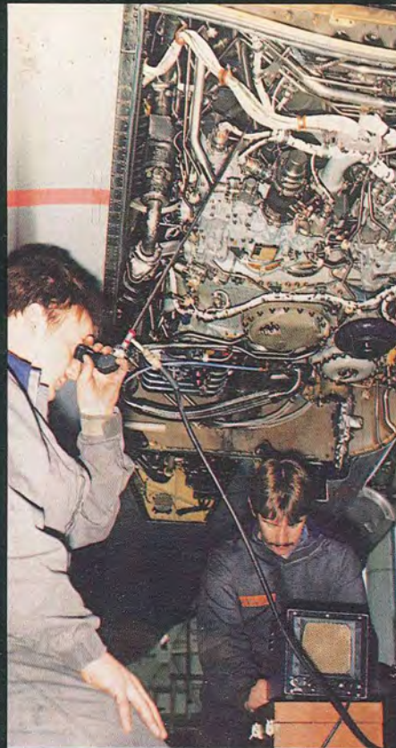
Rotor blades and the combustion chambers can be inspected visually
