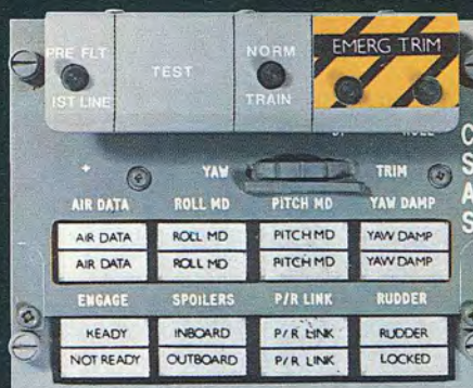
CSAS Cockpit panel with BITE functions and failure indications
