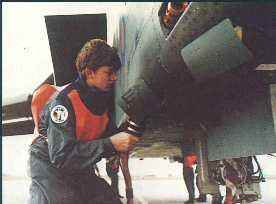
AC Ground supply to save APU life
