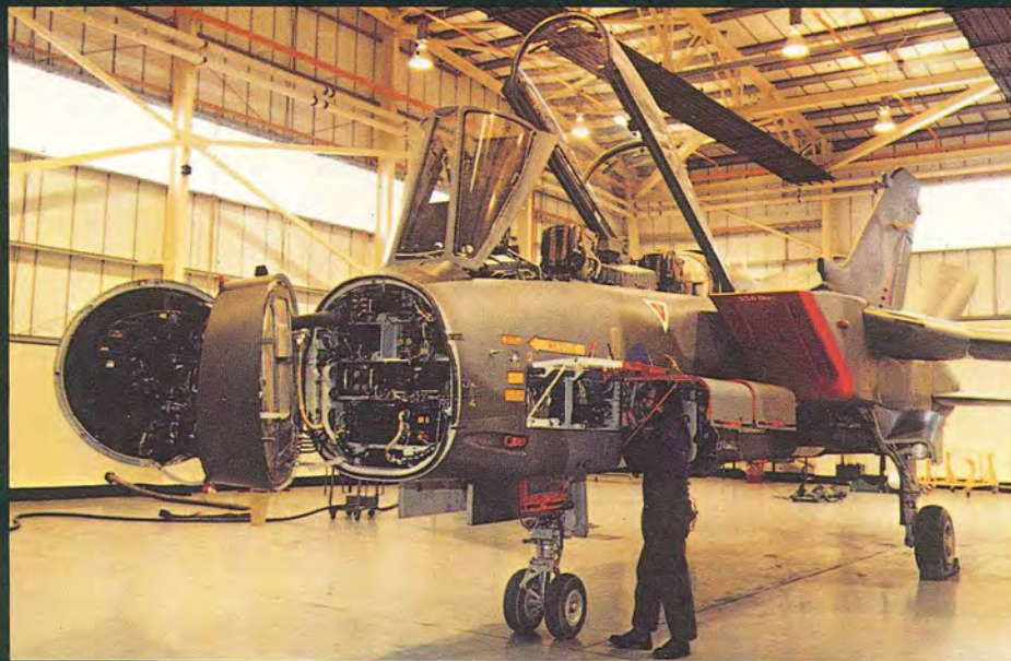
Over 350 easily removable panels provide access for maintenance work
